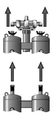
Remove check valve block
