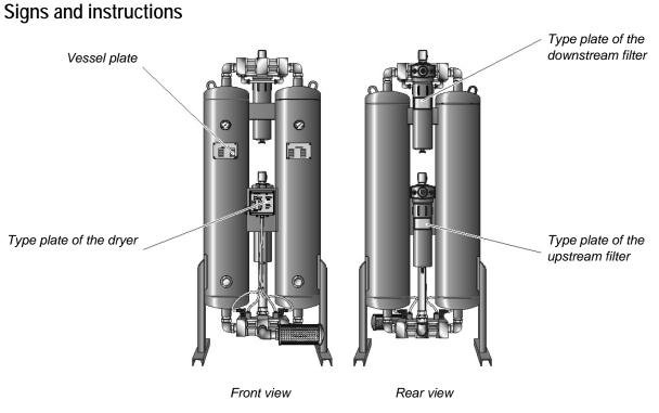
Please note the above plates and instructions attached to the dryer. Ensure that they are not removed and are always readable.
