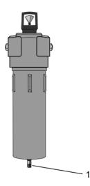
If no compressed air or an unusually large amount of condensate, or no water condensate at all, emerge, you have to remove the condensate trap, clean and if necessary, replace the same. To this end, proceed as follows:
