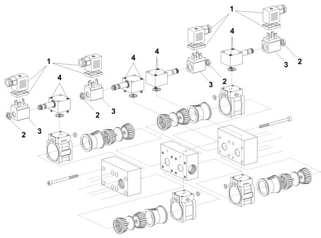
Rear view of solenoid valve block: replacing pilot valves and solenoids
