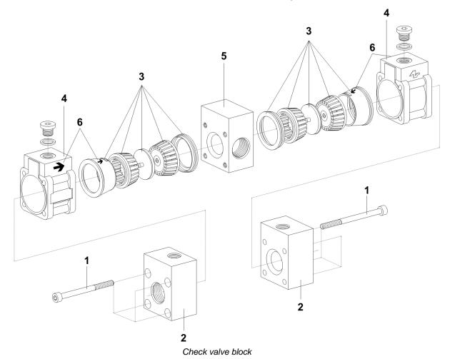
Remove the screws (1) from the threaded blocks (2, 5).
