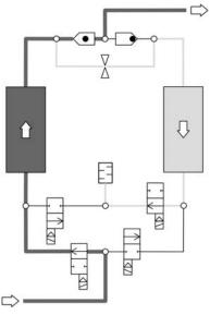
Here, adsorption is shown in the left vessel.
