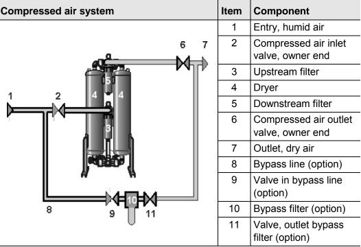
Example of an installation with bypass line
