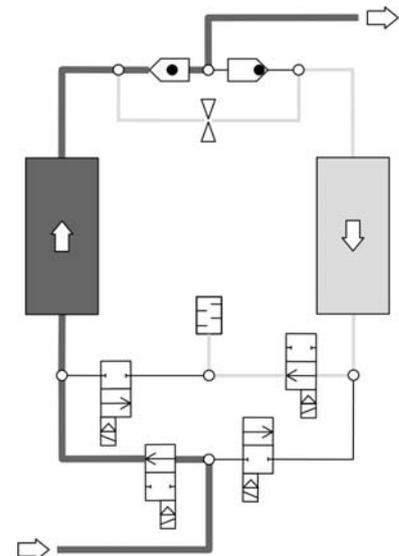
*Here, adsorption is shown in the left vessel.*
